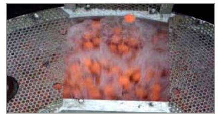
WWETCO Filter media after 30 minutes of low flow rate backwashing.
