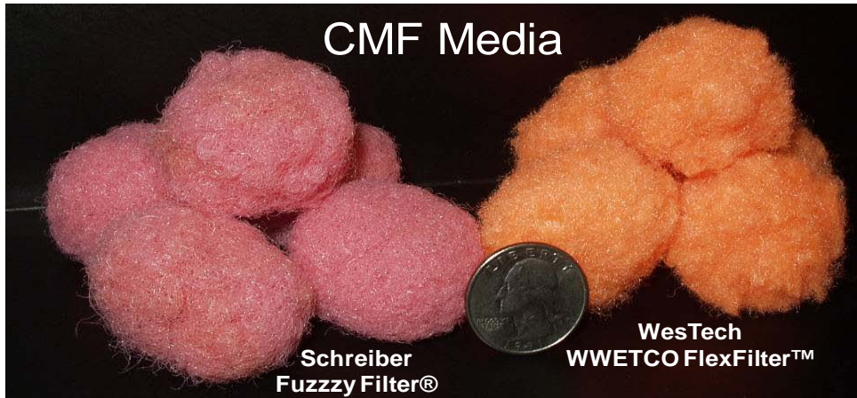
Figure 2. Compressible media filtration relies on a bed of synthetic fiber spheres to filter pollutants from the liquid stream.
